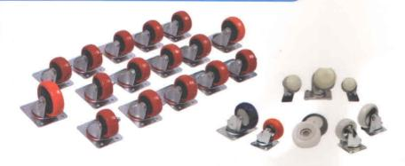
We make Different Type of Castors. Specially Developed Dust Free Swivel Castors have pressed Zinc Steel Body with Thrust bearing for Swivel Movement and Axial ball bearing. High Impact Nylon (Also Polyurethane) wheel provide smooth and silent movement of the Card can. It is available in 60 mm and 80 mm size. We also make customized castors.
