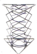
Galaxy Springs are manufactured from High Carbon Spring Steel on Fully Automatic Machines. The Heat Treatment is done with PLC Controlled Automatic Temperature Control Furnaces, to give Perfect Load and Pre Tension. Spring are Tested and supplied with Different load barring capacity as per customer requirement.
